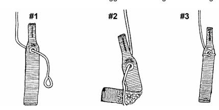
Route the steering line through the slider, then the toggle guide ring and then the toggle. **See drawing #1.** Thread the toggle through the loop in the steering line. **See drawing #2.** Pull loop up to the toggle grommet. Note that the loop of the steering line is going through and around the toggle. **See drawing #3.**
