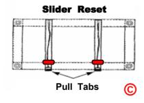
This is best accomplished by grasping the bar tacks located at each end of the channel and pulling them apart. Make certain to extend the slider back to its full length, with the pull tab seated against the stop buckle.
